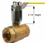
The –XLD extended locking handle is made of robust plated steel and provides additional safety benefits for the user. The handle can be locked in both the open and closed positions. Extension length provides for handle clearance above standard piping insulation thicknesses.
