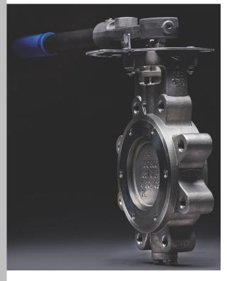
of pressure and the disc should be in between 30 and 70 degrees open. Due to the characteristics of steam, if a disc is positioned less than 30 degrees open, it creates high velocity flow in the area between the disc and the seat. This high velocity steam can pull part of the seat out, which gets crinkled and damaged when the operator tries to close the valve.
