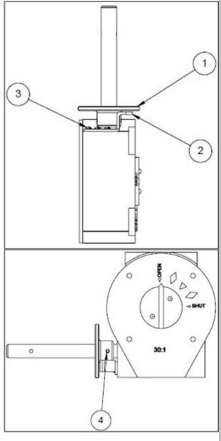
When the installer has properly positioned the disc, they simply put a lock through the wheel and bracket. This will prohibit the handwheel shaft from turning in either direction.
