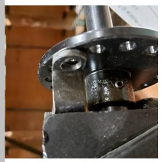
When assembling the optional kit in the field, it's likely that the handwheel will already be on the shaft. That handwheel will need to be removed for the assembly, and then replaced when assembly is complete.
